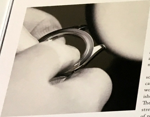
SURFACE FINISHING is carried out by hand to obtain an even, mirror-like polish, here on a steel middle case.
