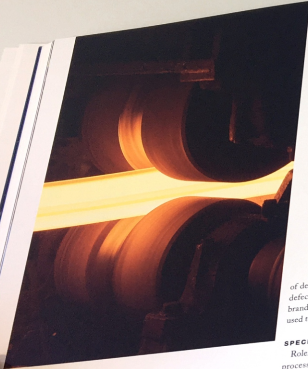
HOT-ROLLING 904L steel billets. OXY-FUEL cutting (right).
